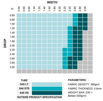
**NOTE:** Using alternative parameters will change the system capacity.
