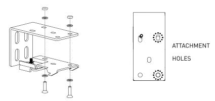
STEP 2 - ATTACH ASSEMBLED BRACKET TO WALL
