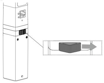
STEP 4 – CHECK THE MOTOR AND BATTERY OR AC MODULE ARE SECURELY ATTACHED BY TRYING TO PULL THEM APART
