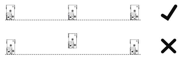
STEP 3 - ATTACH DRAPE TRACK (ASSEMBLED) TO CEILING BRACKETS AND SECURE
